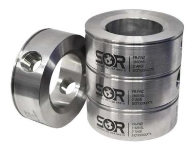
When used as a calibration ring, a known pressure is applied to one of the flushing connections while the attached instrument is cycled through a calibration routine. The SOR 1010FR Flushing Ring can also be installed without flushing connections as a spacer or to provide heat dissipation.
