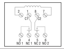
For Type 1520 Flow Detectors equipped with DPDT relays, a wiring schematic and pin position schematic is shown on page 2. When the 1520 is actuated, the coil will energize and "make" both NO1 and NO2 while it will "break" NC1 and NC2. This provides a DPDT circuit.
