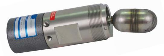
The float moves a magnet into the field of a magnetically actuated pneumatic valve. The pneumatic valve is pilot operated. An amplifying relay provides quick response.
