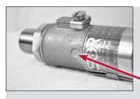
The 815LT can be easily configured externally with a magnet. Simply place a magnet to the targets located on the housing for 3 seconds and set the zero and span.
