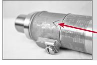
To set the Span, follow the same steps except place the magnet on the triangle on the housing for 3 seconds. Using this method requires a power and a pressure source. Almost any magnet can be used, and SOR can provide the magnetic tool if needed.
