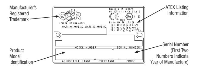
NOTE: The unit conforms to the requirements of clause 6.3.12, EN 60079-11: 2007. The unit is capable of withstanding a 500 Vrms isolation test between circuit and enclosure.
