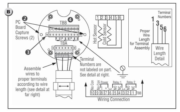
NOTE: Connections to sensors are factory installed and should not be disconnected in the field.
