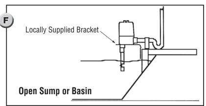
NOTE: The instrument must be positioned so that overflow does not flood electrical housing (see F)
