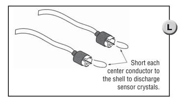
connector so that the center conductor and outside shell make contact. (See (L))
