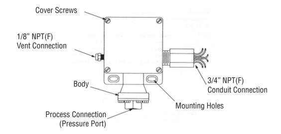
**Mounting Hardware** Fasteners per SOR Test Report 9058-102 consist of two 1/4-20, Grade 5 screws (not supplied). Torque screws to 70 to 85 in-lbs.
