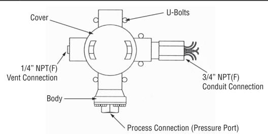
**Mounting Hardware** Fasteners per SOR Test Report 9058-102 consist of three standard grade 1/4-inch U bolts (not supplied).
