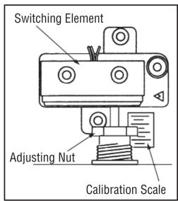
To adjust pressure at which switch will operate, remove cover and tighten the hex head adjusting nut with a 3/4" wrench to increase pressure; loosen to reduce pressure. Sighting across the top of the 3/4-inch hex adjusting nut to the scale gives approximate set point pressure.
