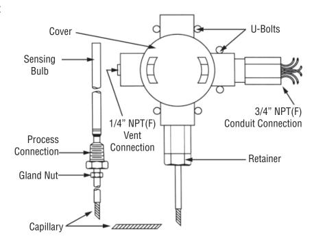
**Mounting Hardware** Fasteners per SOR Test Report 9058-102 consist of three standard-grade 1/4-inch U bolts (not supplied).
