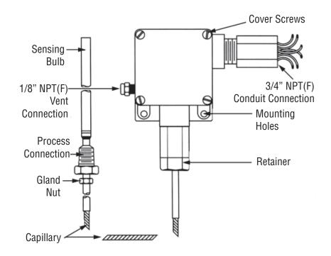
**Mounting Hardware** Fasteners per SOR Test Report 9058-102 consist of two 1/4-20, Grade 5 screws (not supplied). Torque screws to 70 to 85 in-lbs.
